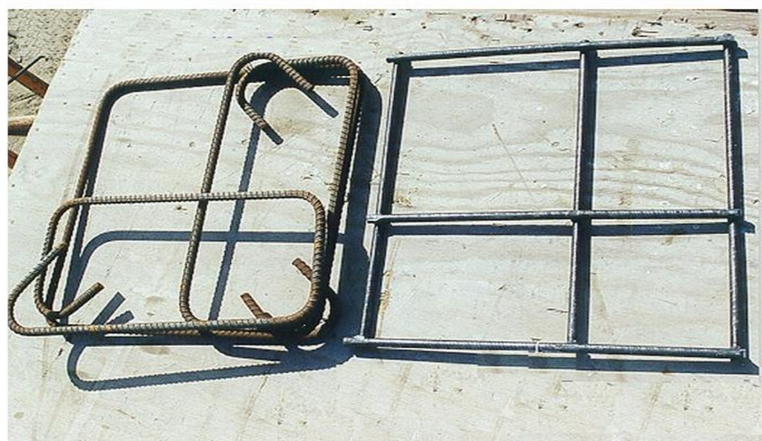
Left: Conventional confinement reinforcement with protruding hooks and \pm 12.7\text{mm} dimensional tolerance
